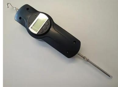
**Figure 4.** Digital dynamometer for force measurement PROTESTER WDF-30
