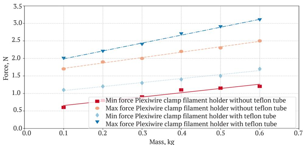
Figure 9. Clamp filament holder force to mass comparisons using Plexiwire plastic spools
